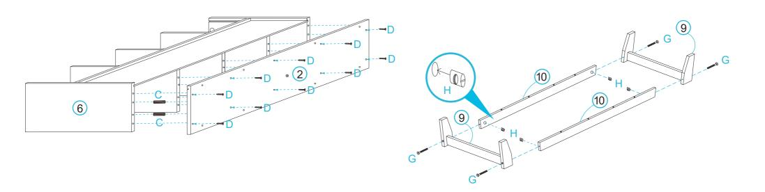
Insert10 xdowels (C) into panel [2]. Attach panel [2] to panels [5], [6] and [2] and secure with 10 x long screws (D). Tighten with a screwdriver.
