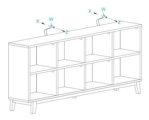
Move the unit into the desired location up against a wall, do not drag. Use a drill to create a small hole lining up with the top of the 2 x safety strap (W) and secure with 2 x wall anchor (X), 2 x washer (Z) and 2 x long screw. Tighten with a screwdriver. Ensure the unit is balanced and steady before use. You're done, enjoy!
