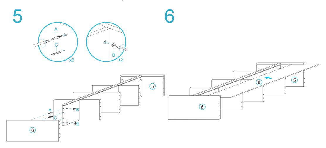
Screw in 2x bolts (A) and insert 2x dowels (C) into holes in panel [6]. Slot together with the rest of the structure as shown. Place 2x locking nuts (B) into holes in the panels and tighten with screwdriver.
