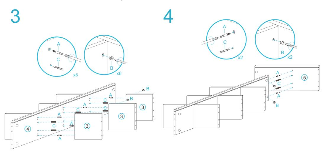
Attach panel [3] into panel [4] and secure 6 x bolts (A) and 6 x dowel (C). Slot together with the rest of the structure as shown. Place 6x locking nuts (B) into holes in the panels and tighten with screwdriver.
