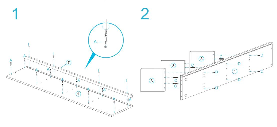
Insert 10 x bolts (A) into panel [1]. Attach panel [7] into panel [1] and secure with 4 x long screws (I). Tighten with a screwdriver.
